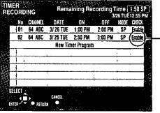
Displayed if the recording can fit in the remaining space on the disc.
